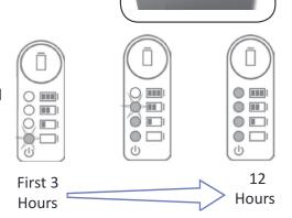
**NOTE:** In the case of a power cut, switching the power socket off or disconnecting the charging lead the charging process will not be interrupted as the unit remembers the previous charge state.
